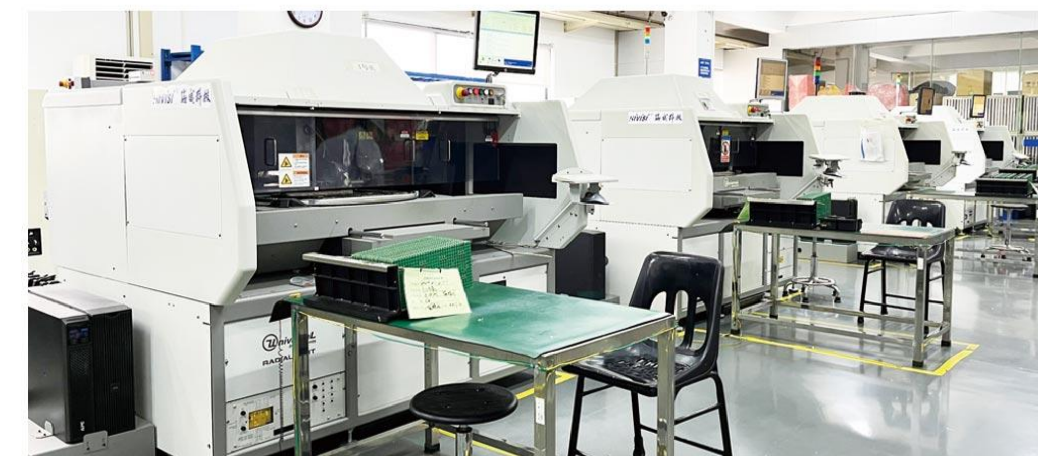
环球自动插件机 Univeral automatic through hole mounting machine
