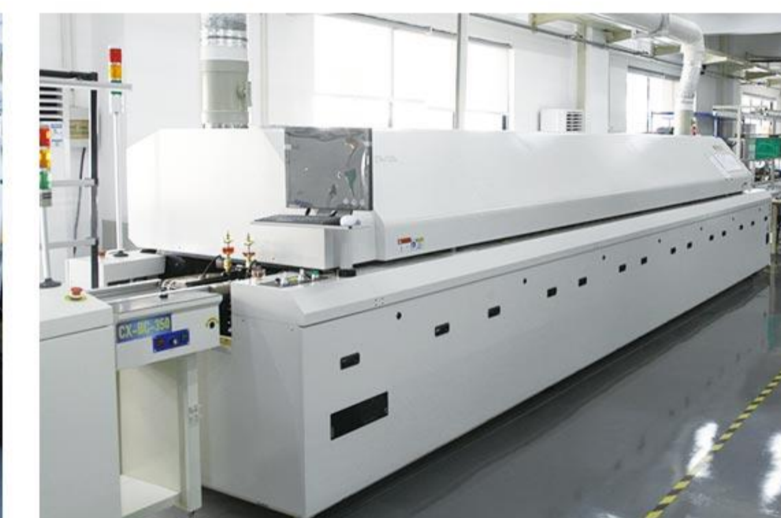
劲拓12温区回流炉 Reflow soldering machine with 12 temperature zone
