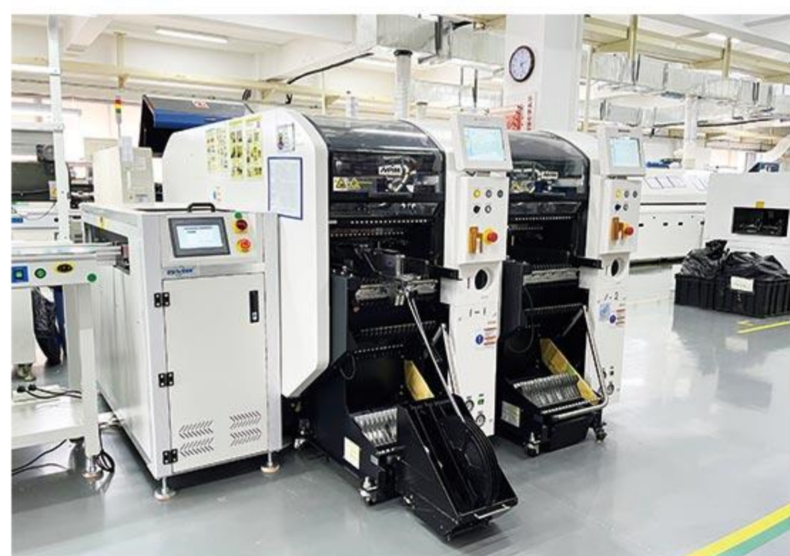
松下高速贴片机 Panasonic high-speed chip mounter
